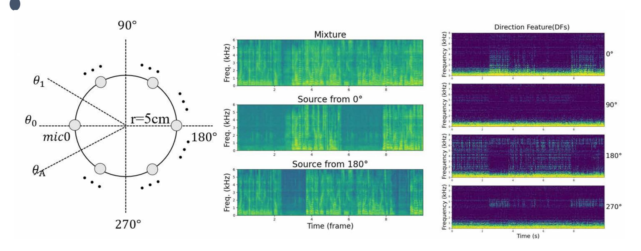
Cosine similarity between ideal phase difference and target-dependent phase difference Target directions degree 0 and degree 180 more discriminative features from 1kHz – 8kHz
