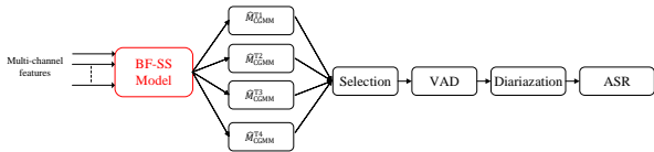
Figure 3: An illustration of the whole framework for multiple-array diarization and recognition track.
