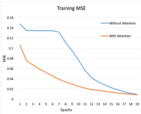
Figure 4: Training MSE curves for the vanilla system along with the proposed attentive network.
